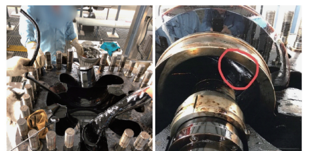
图 3 从某输油泵中取出的异物和其叶轮出现的裂纹 Fig. 3 Foreign matter removed from the oil pump and cracks on its impeller
