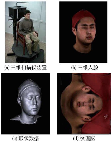
图 2 Cyber Ware 扫描仪及其获得的三维人脸数据 Fig. 2 The Cyber Ware scanner and 3D face data acquired using this device
